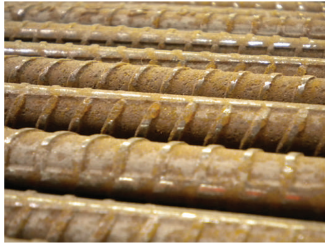
Figure 3 – The "heavy" rust on the bars is tight and does not alter the deformations. The surface is acceptable and cleaning is not required.
