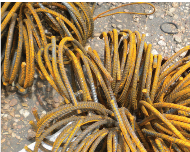
Figure 2 – Although these hoops look fairly rusty, this rust is superficial and has no impact on bond behavior.
