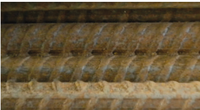
Figure 7 – The tight rust has not altered the deformations on the #9 bar surface.
