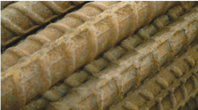
Figure 6 – Tightly adhered rust on a bundle of #9 bars left exposed to normal atmospheric conditions for 22 months.
